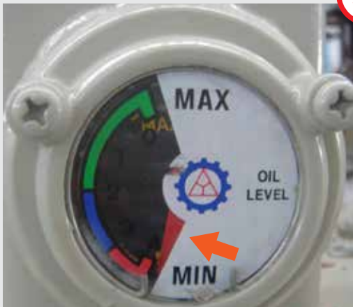
Oil Level Indicator indicating oil level below normal level
